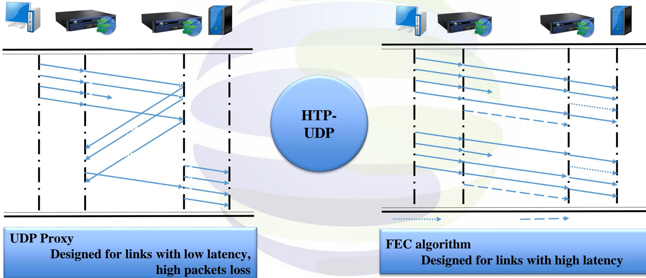
HTP(UDP packet) is based on UDP design for high packet loss environment
