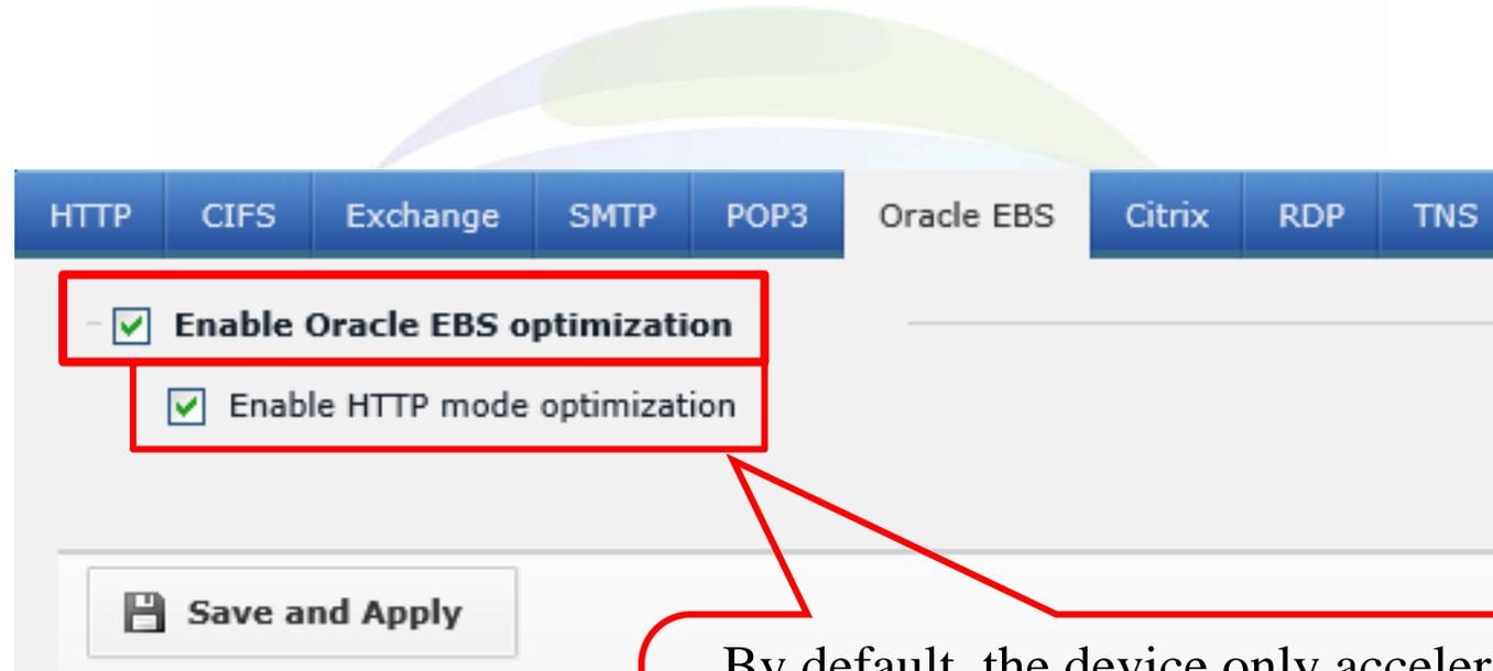
By default, the device only accelerate Oracle EBS socket mode. Once this option is checked, the HTTP mode Oracle EBS will be able to accelerate.
