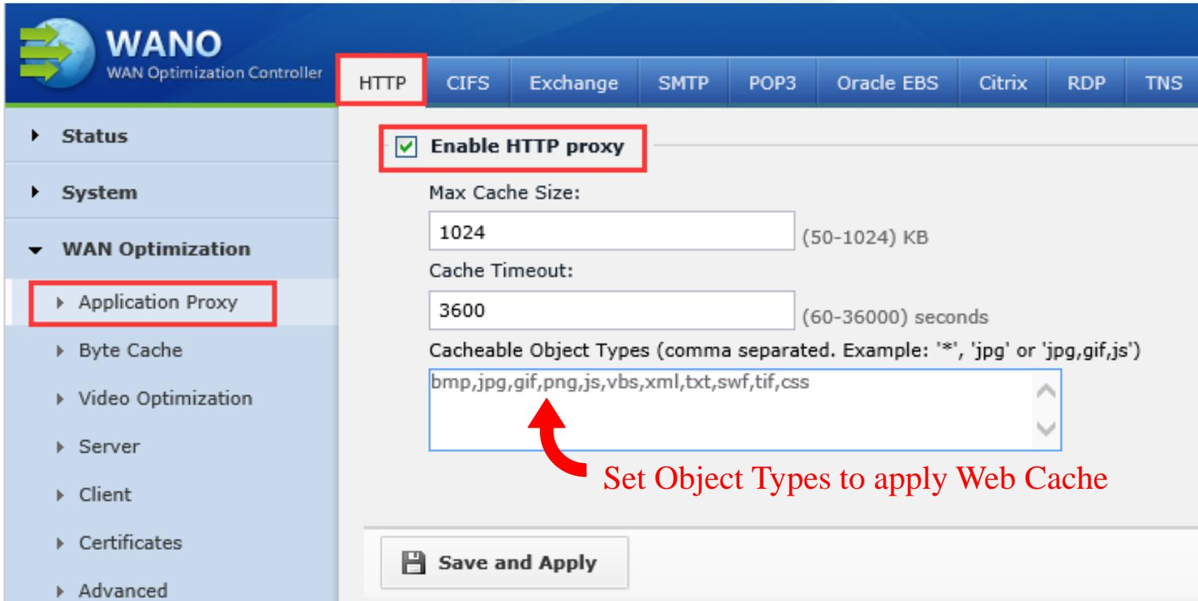
The screenshot shows the WANO WAN Optimization Controller interface. The left sidebar contains a navigation menu with the following items: Status, System, WAN Optimization (expanded), Application Proxy (highlighted with a red box), Byte Cache, Video Optimization, Server, Client, Certificates, and Advanced. The main content area is titled 'HTTP' and contains the following configuration options:
