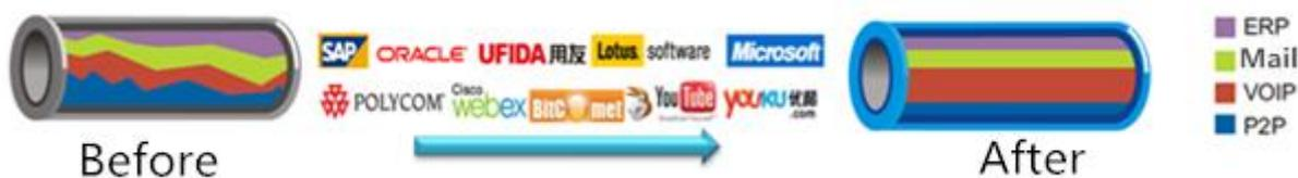
**Optimization:** Video conference is a instant messaging application, use UDP protocol transmission, but UDP is not a reliable protocol, it is easy to has packets loss issue. HTP-UDP is a optimized protocol for UDP traffic by Sangfor, it used for reduce packets loss especially for video conference.
