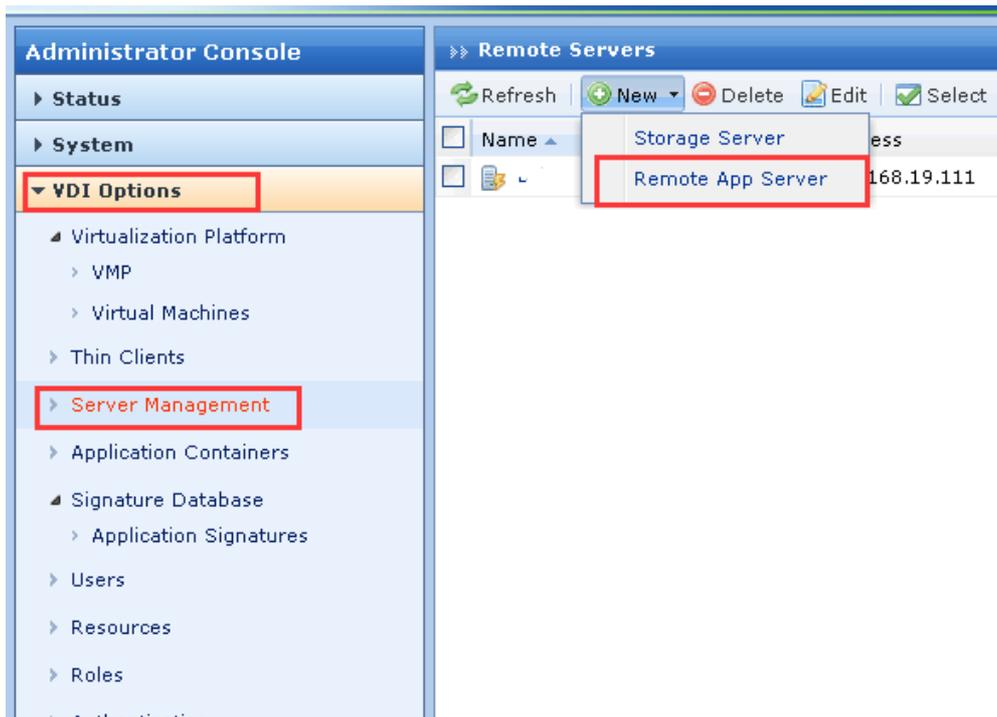
Fill in the Remote App Server name, Windows Server IP address, username and password, and click "Test Connection" to test the connection with the terminal server.
