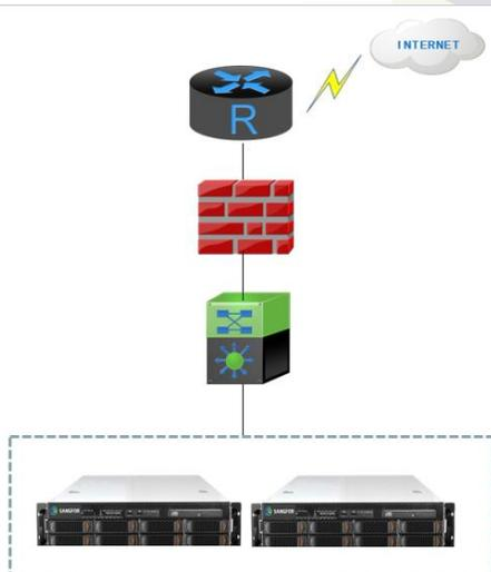
Instead of using traditional IT infrastructure, Sangfor HCI puts resources into commodity servers. One cluster can provide compute & storage resources, and management is unified into one single web platform, with NFV features that can be enabled any time without adding new hardware.
