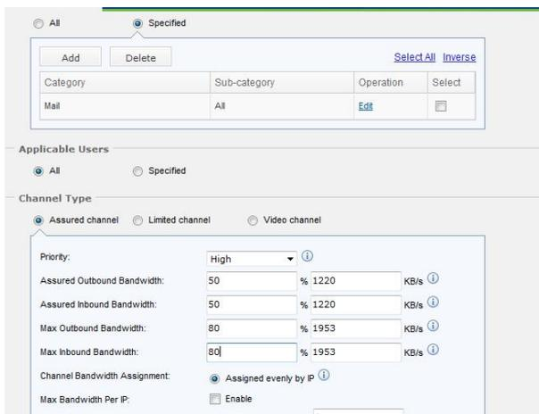
12. Add a bandwidth control policy chose P2P/download tool application , use limited channel, Max bandwidth 80%, Max bandwidth per IP 100KB/s.
