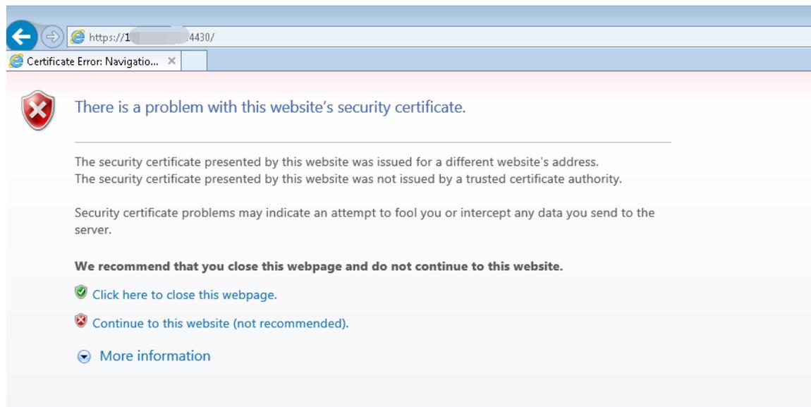
Everyone knows that when accessing the VPN login page is using the https protocol. Normally if accessing to device and the device certificate is not trusted, means that endpoint fails to verify the server certificate. The endpoint will think that the connection to this server is an insecure connection, so this warning box will pop up. Sangfor device usually uses the method of updating the device certificate to remove the warning.
