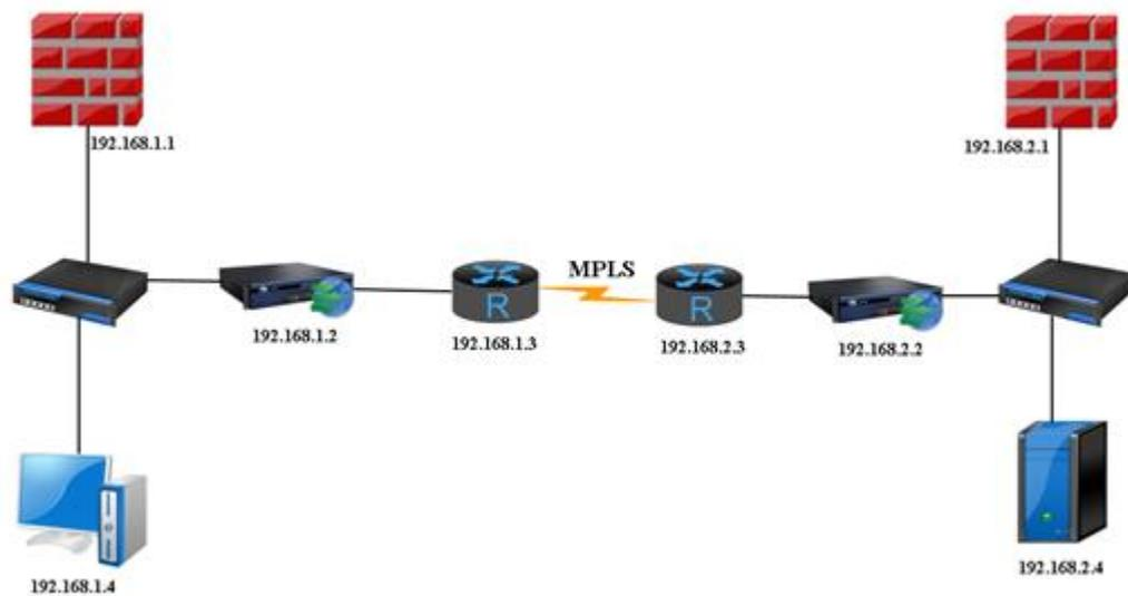
The WANO (IP address: 192.168.1.2) deployed as Bridge mode, the WAN interface is connected to the Router (IP address: 192.168.1.3) and the LAN interface is connected to the Switch. The default gateway of the WANO is IP address: 192.168.1.1.
