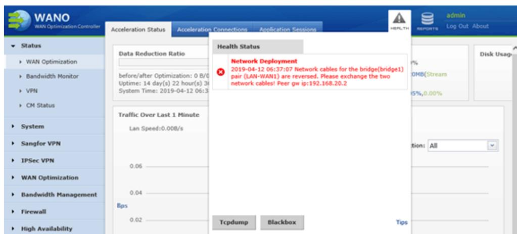
Firstly, ensure the network cable connection is normal. If it is reversed, unplug and plug with the correct way. If the network cable connection is normal, means it could be caused by incorrect Gateway IP set in the deployment.
